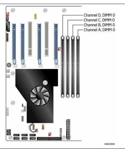
Figure 3. Memory Channel and DIMM Configuration
